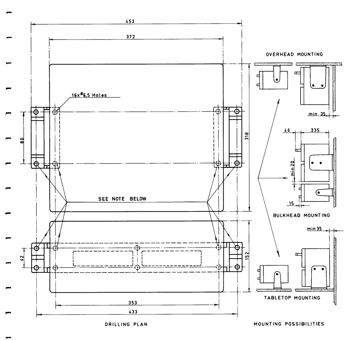
NOTE: CU 6000 BRACKET MAY BE USED AS A JIG FOR THE MARKING OF TU 6X00 BRACKETS HOLES AS SHOWN.
