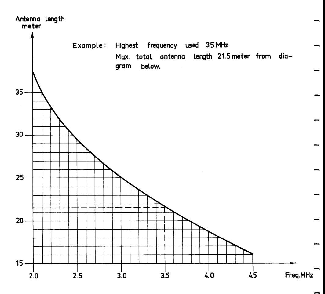
Max. Antenna length versus frequency with the shortening capacitor inserted.
